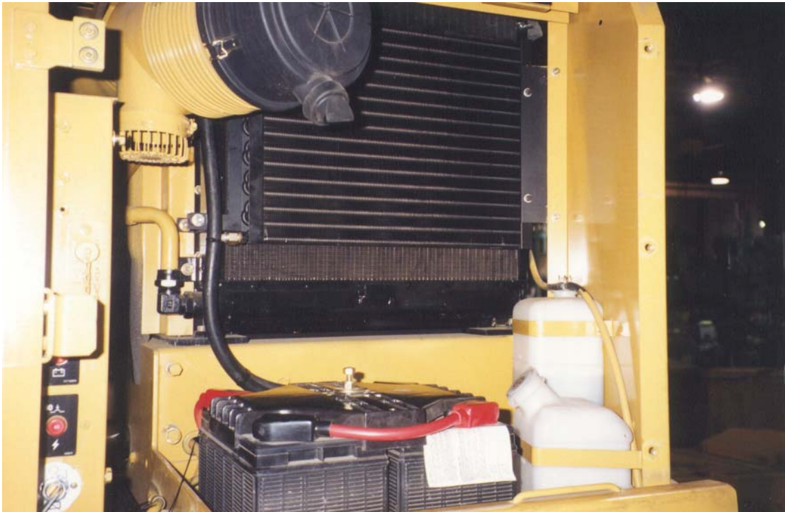
View of condenser in place on radiator.
