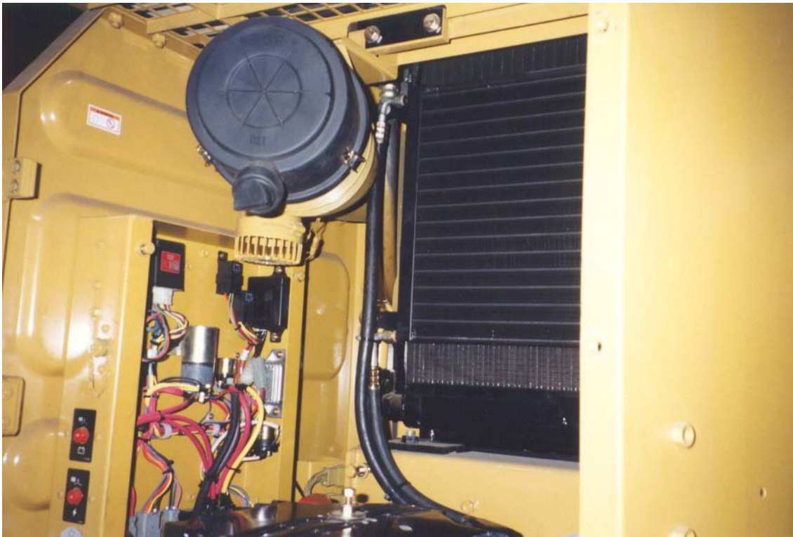
Fitting side of condenser in place.
